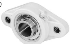
These Thermoplastic units are equipped with TRITAN Stainless steel inserts. The rings and balls are constructed of AlSI 440C martensitic stainless steel and retainer, slinger & seal frame and the set screws are constructed of AlSI 302 austenitic stainless. The inserts are lubricated with H1 USDA/FDA Food Grade grease.
